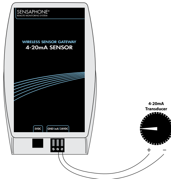
4-20mA Transducer using 24VDC power supply
